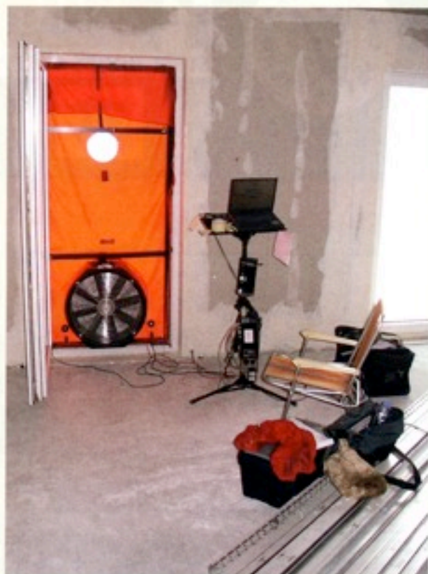
A blower door test (above left) is a mandatory requirement for all certified passive houses; insulation detail (above right) around a well insulated window in a passive house
